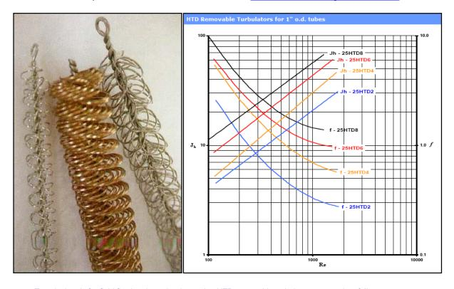
To calculate hi for fluid flowing through tubes using HTD removable turbulators proceed as follows:
