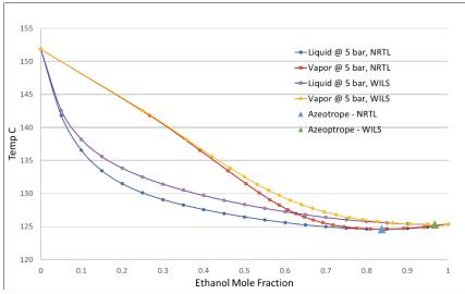
Figure 1 - Txy Chart for Ethanol / Water mixture at 5 bar
