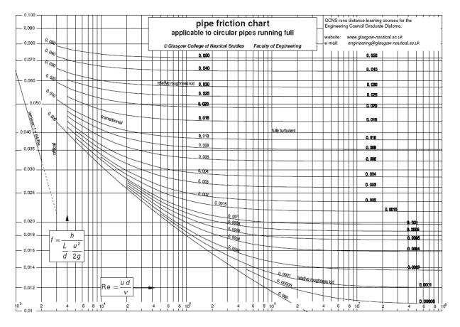
Example Friction factor for cast iron pipe D = 500mm,  $\varepsilon$  = 0.5 mm ( $\varepsilon$ /D = 0.001) with Re of 300000 is 0.026
