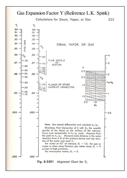
The sizing procedure is to determine an initial S and then d/D assuming  $F_c = 1$  and Y =1. Then use alignment chart to determine Y and obtain new d/D from modified S/Y value.
