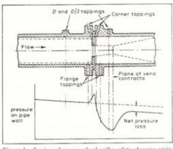
Figure 1—Section of square-edged orifice plate showing variation of pressure along the pipe wall (by courtesy of BSI)
