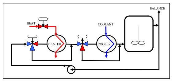
This arrangement requires an adequate recirculation flowrate determined by the reactor size and number of mixing nozzles. The jacket inlets have mixing nozzles fitted to induce a rotational flow in the jacket and enhance heat transfer. Nozzles should be fitted to induce circulation in the same direction of rotation. Inadequate flow and / or high viscosity at low temperatures will result in poor heat transfer and could result in loss of thermal stability when carrying out exothermic reactions.
