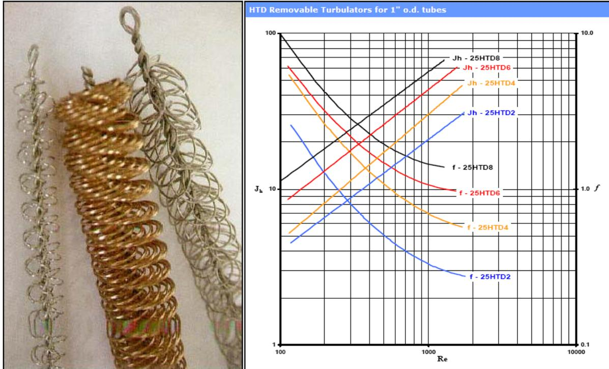
To calculate  $h_i$  for fluid flowing through tubes using HTD removable turbulators proceed as follows:
