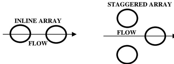
Triangular pattern provides a more robust tube sheet construction.
